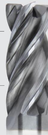
Proprietary end face design — Twisted cutting edge increasing the corner stability, enabling soft cutting action even at highest ramping angles.
