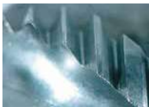
Cutting Edge after Tapping 1,000 Holes
