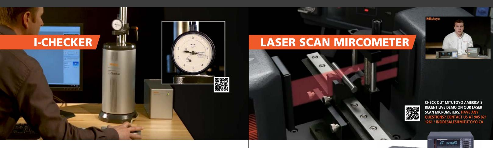
Inspect your indicators with Mitutoyo's I-Checker Instrument for efficient in-house calibration. The I-Checker can be used on various indicators such as Dial, digimatic and dial test. Also used for calibration of Bore gauges.
