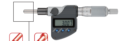
Equipped with a non-rotating device 350-261-30 (Stem dia. 12 mm, water-proof type) Mass: 235 g
